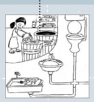
...the water from washbasins is redirected to the flushes and the solid waste is dumped into pipes running under the basement...
